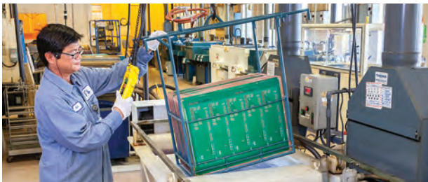
Uyemura KAT ENIG line at ITL Circuits
