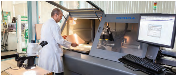
Dual UV and CO 2 Cobra laser for micro-via drilling, die cavity ablating and flex circuit profiling
